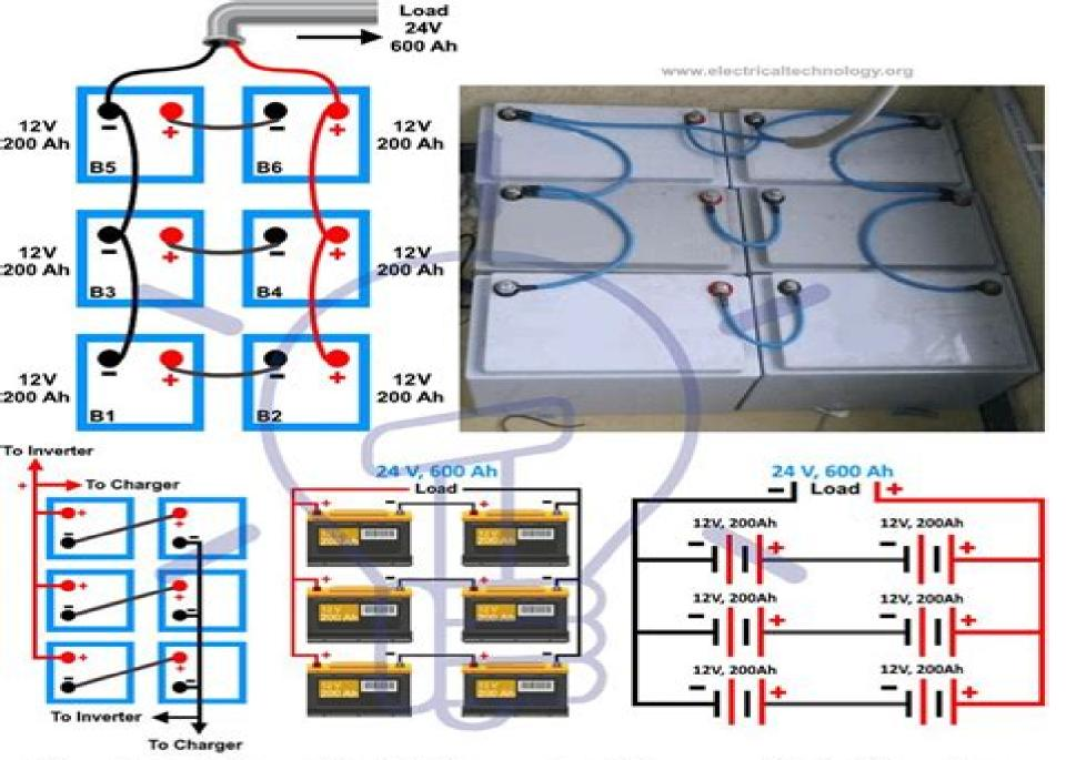
Series-Parallel Connection of Batteries
