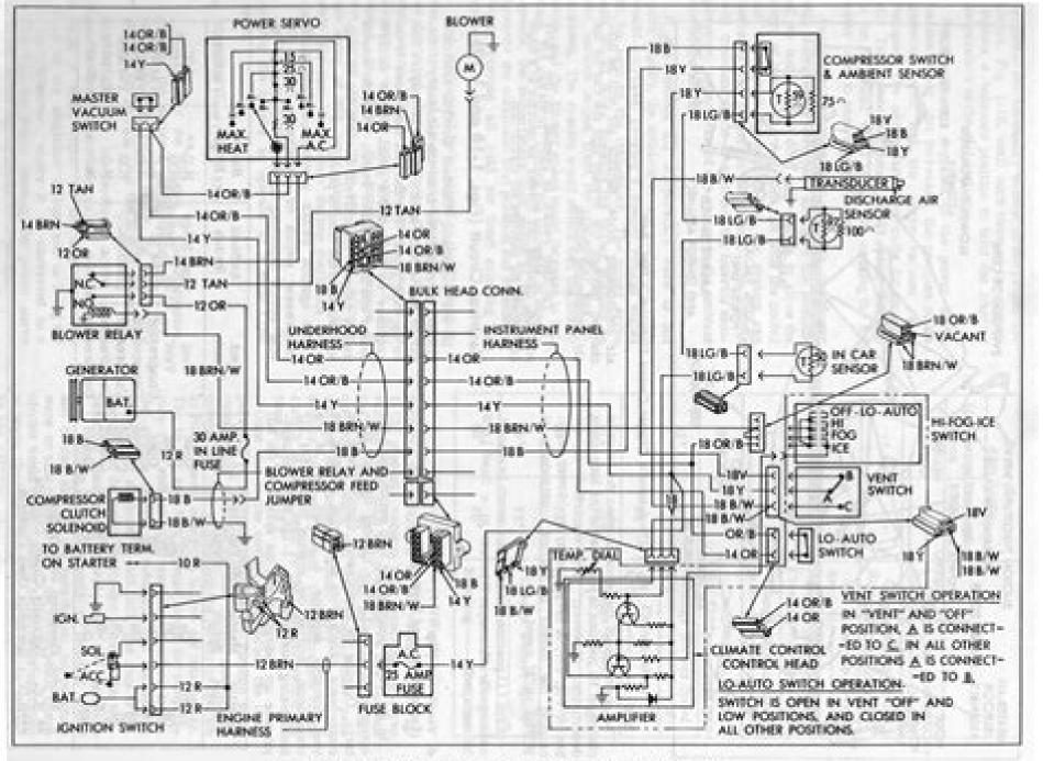
Fig. 1-19 Automotic Climate Control Circuit Diagram (Except 693 & 697)
