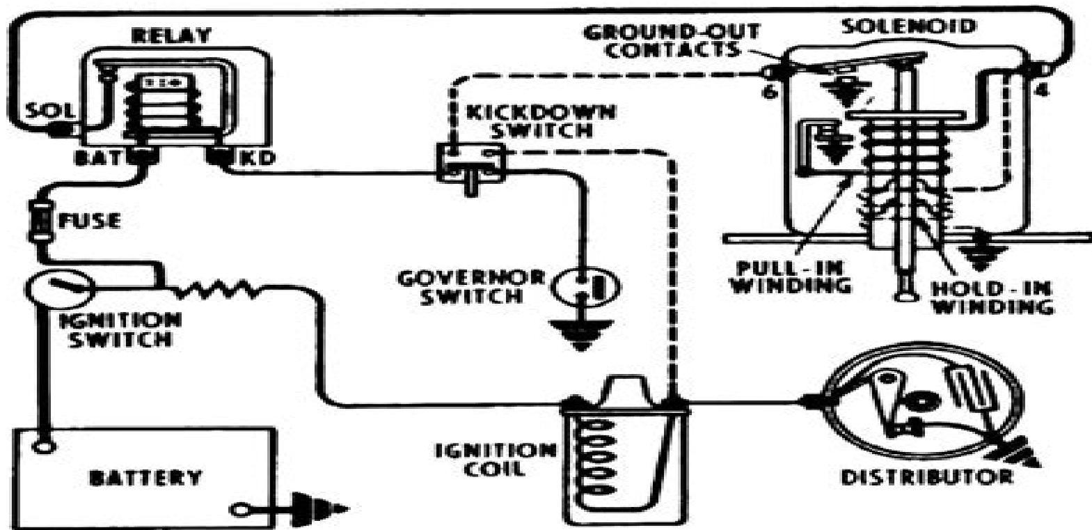
Overdrive Electrical Circuit Wiring Diagram
