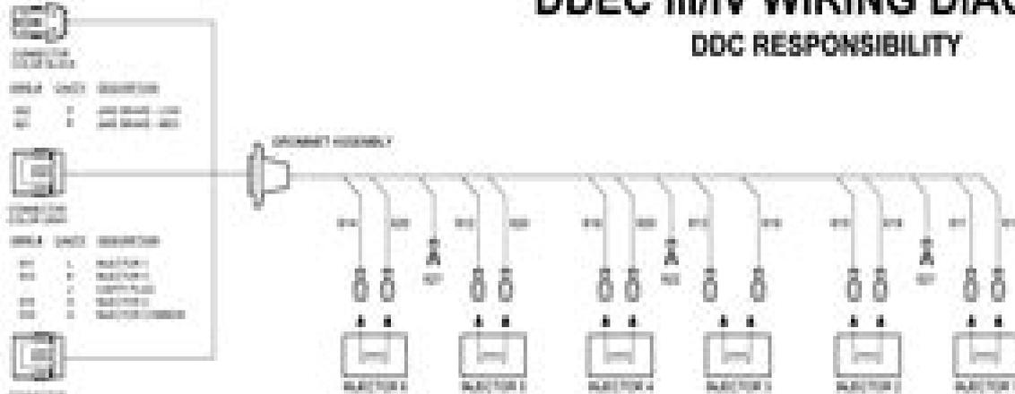
INJECTOR HARNESS SCHEMATIC (SERIES 60 WITH JAKE BRAKES SHOWN)
