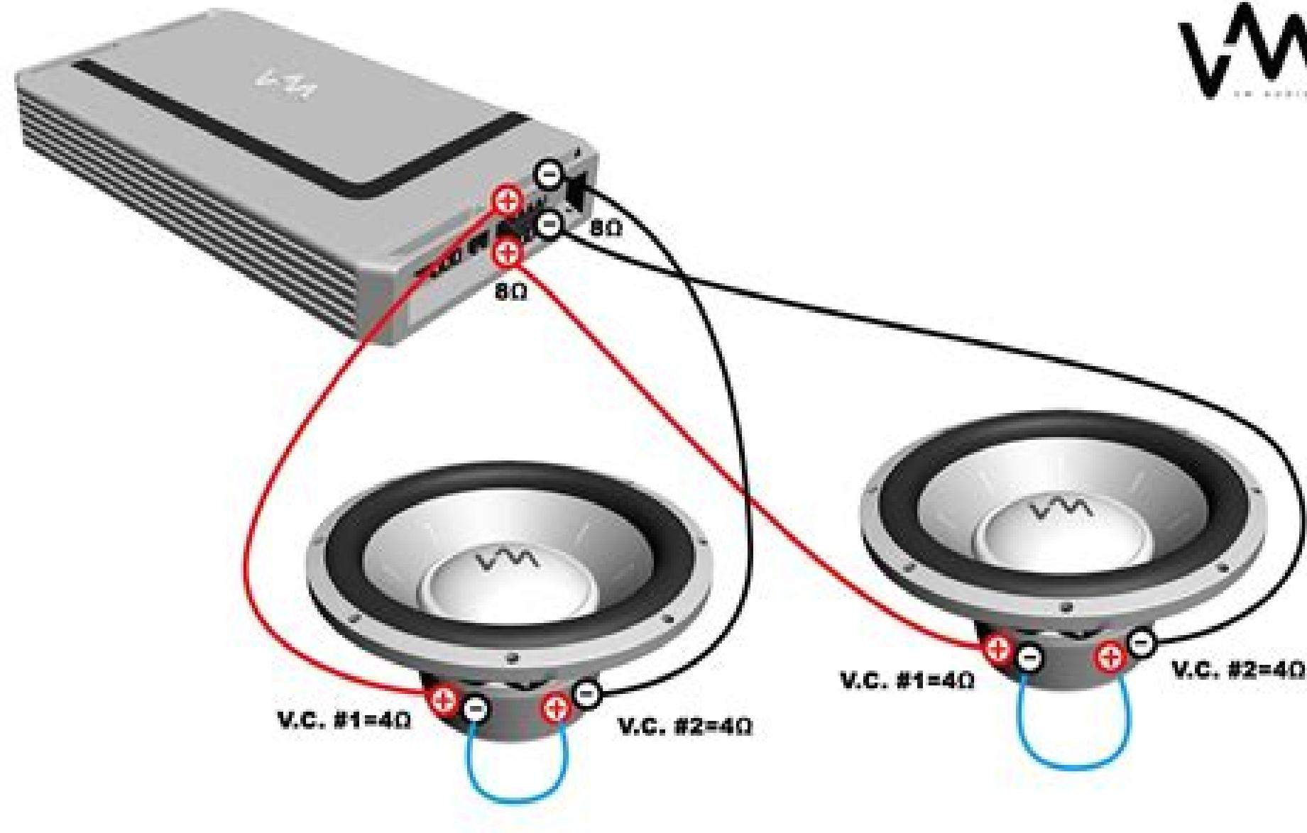
TWO 4Ω DVC SUBS, BRIDGED 4-CHANNEL AMP: 2 X 8Ω LOAD
