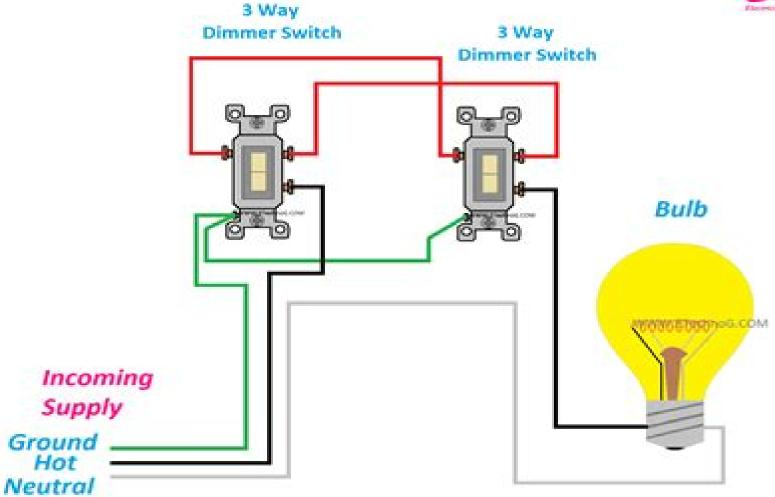
3 Way Dimmer Switch Wiring Diagram
