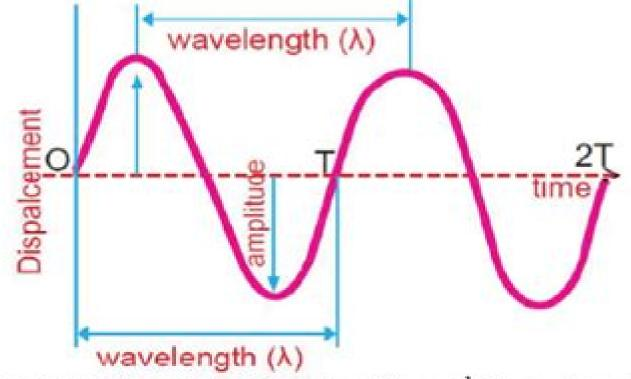
The *frequency* is related to the period and has units of Hz, or s<sup>-1</sup>. The number of such oscillations per unit time is the frequency of the sound wave.  $v = \frac{1}{T}$
