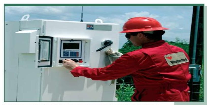
Continuous pump-fill control with speed and torque override for optimum management of rod-pumped wells.
