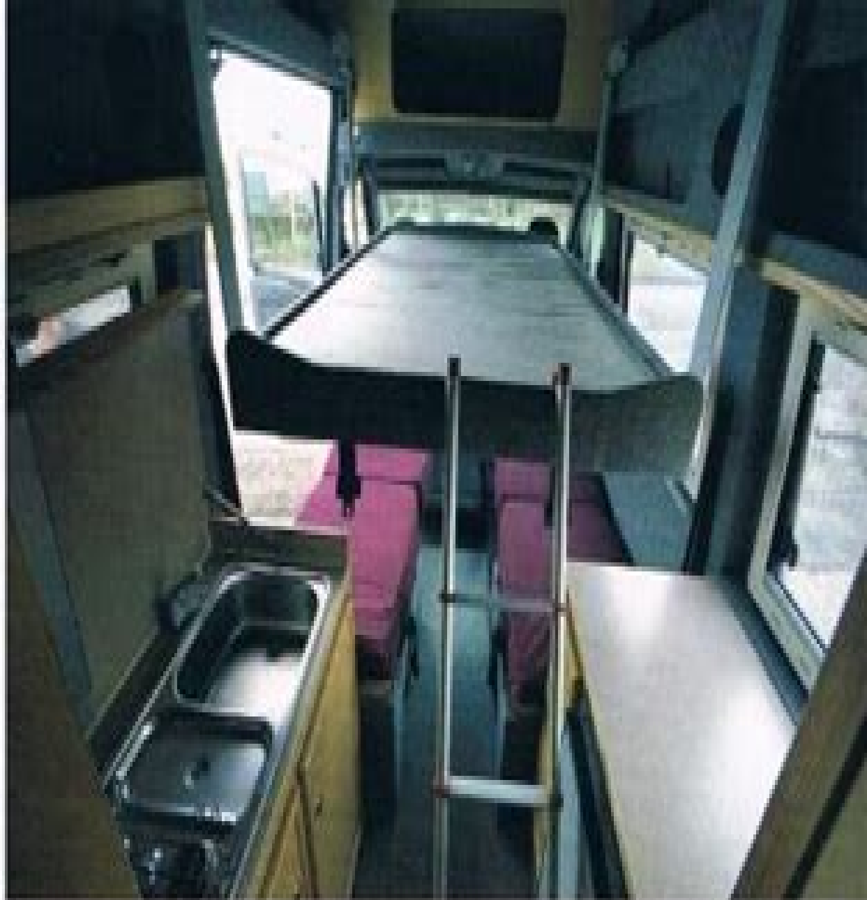
Youngs designed and built this roof bed specially for this Renault Master conversion. The occupants can use their reading lights without disturbing those in the beds below
