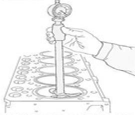
Perform the measurement crosswise at the liner top end, lower end and middle.
