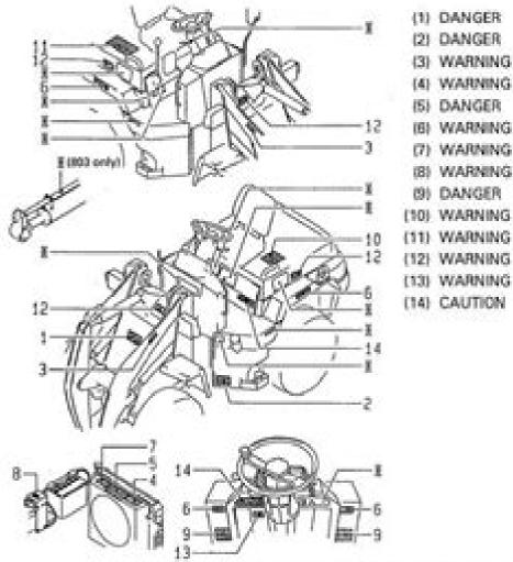
Notes 1: Decals numbered 1 thru 14 are given to provide important safety messages and those marked \* are for the instructions of operation and maintenance and the information about the model number and others.
