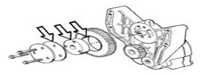
Oil the bearing with engine oil and install the idler gear on the new oil pump.
