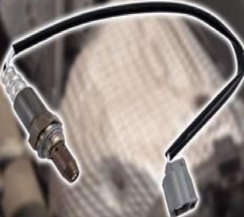
**HOW TO REPLACE UPSTREAM O<sub>2</sub> OXYGEN SENSOR
