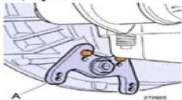
Position the marks on the camshaft which indicate the number of the cylinder to adjust between the marks on the camshaft front bearing cap.
