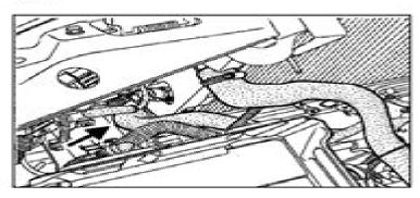
Remove the air filter unit.
