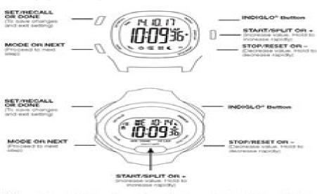
When setting, each button has a different function as indicated above. Watch face will indicate when button changes function.
