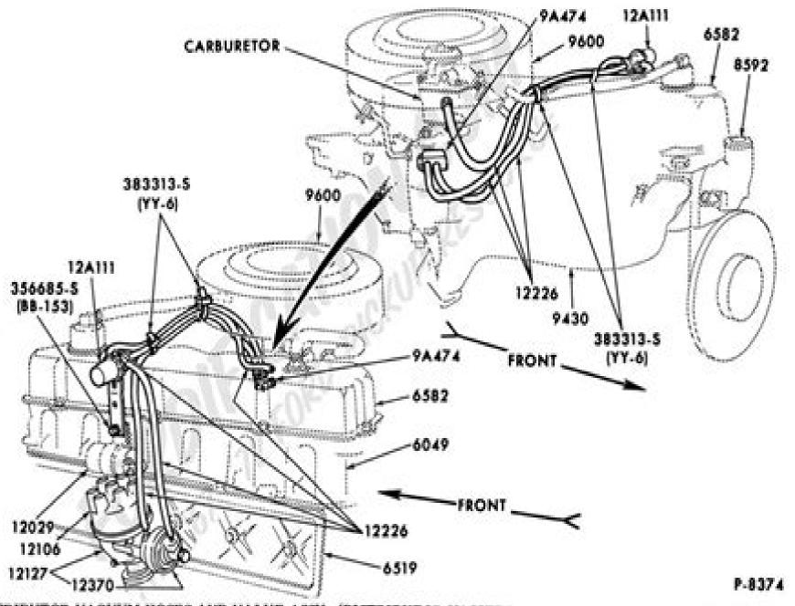
DISTRIBUTOR VACUUM HOSES AND VALVE ASSY. (DISTRIBUTOR VACUUM ADVANCE CONTROL) - 6 CYLINDER 240
