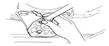
Install the oil supply pipe on the pump and the cylinder block,
