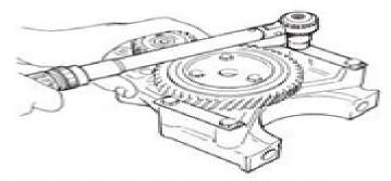
Screw the bearing cap to the oil pump bracket. Torque the screws (65 Nm (6.5 kpm) and lock with the lock tabs. 7
