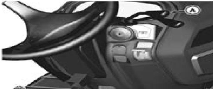
2. Start engine, and pull back top hydraulic lever (A) to raise lift arms to highest position.
