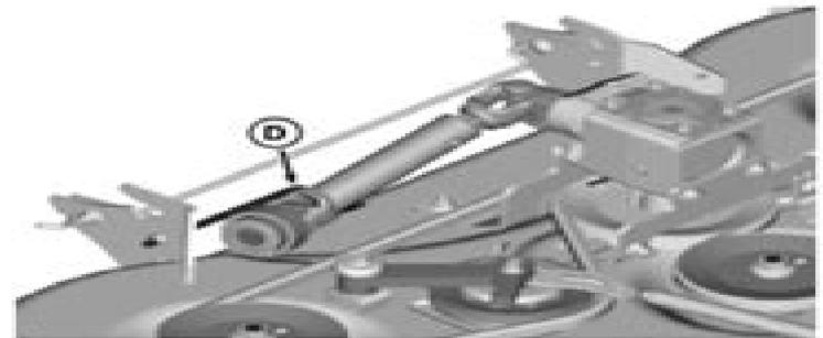
5. If using a standard PTO shaft connection, ensure that PTO shaft on deck is positioned on hanger (D). Make sure that it is clear of where the rear draft arms fit into rear brackets on deck.
