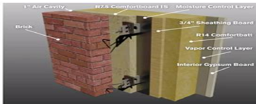
Figure 6: This code-compliant wall is modeled for the Chicago climate. Note: Insulation depicted is comprised of mineral wool R7.5 continuous sheathing board and R14 batt.
