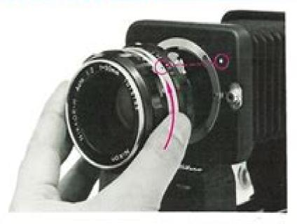
Position the lens in the bayonet mount on the lens panel, lining up the black dot on the lens with the white dot on the lens panel. Then twist the lens counterclockwise until it clicks into place.
