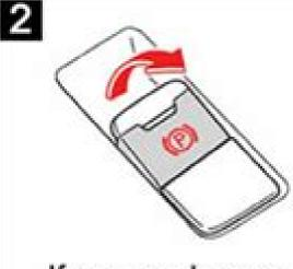
If your car has an electronic parking brake, pull the switch up
