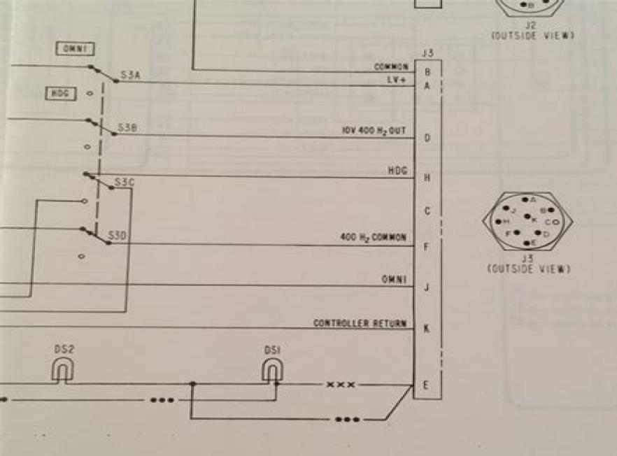
6-1. C-394A Controller-Amplifier, Schematic Diagram
