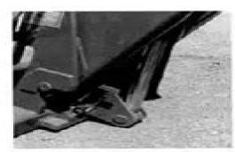
3. Engage Quick Switch (attachment tilt lever bockword).
