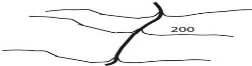
The figure above shows a stream in the center, and three contours crossing the stream. If the contour interval is 50 feet, label the two unlabeled contours.
