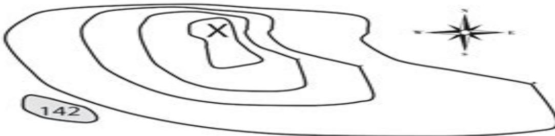
If the contour interval is 50 feet, label each topographic line on the figure above. Note there is a lake in the bottom left of the figure with an elevation of 142 feet, and a mountain peak where the "X" is on the map.
