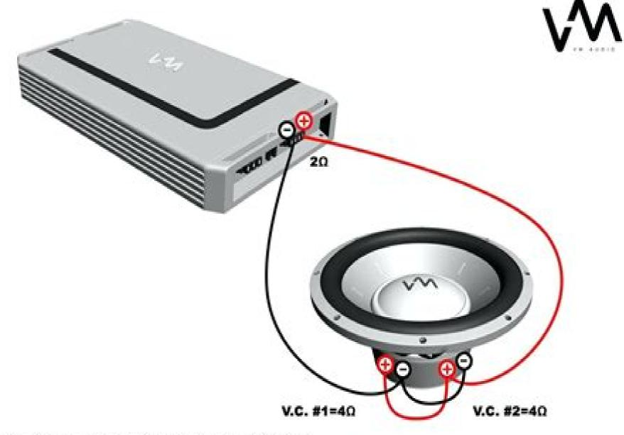
ONE 4Ω DVC SUB, BRIDGED 2-CHANNEL AMP: 2Ω LOAD
