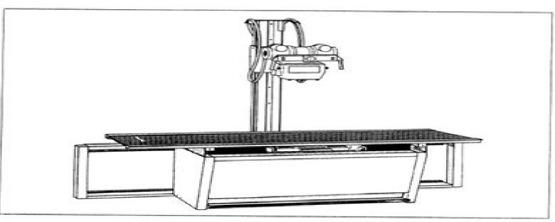
Bucky table with integrated stand for tube assembly
