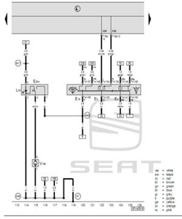
Turn signal switch, headlight dipperiffasher switch, parking light switch, tank filler flap remote release switch, tank filler flap release motor
