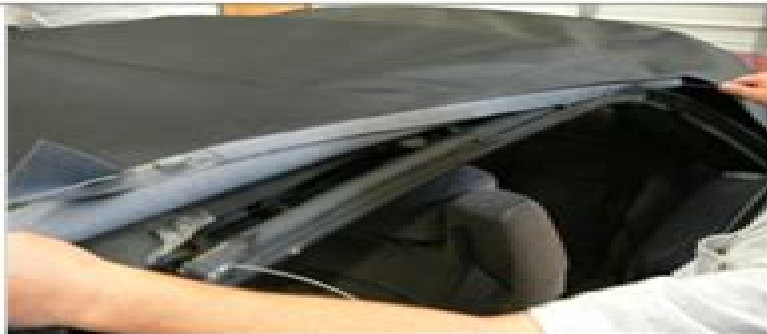
Step 23: INSERT SIDE CABLES Insert side cables from front of top side pockets and screw in back end with spring to frame.
