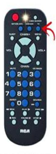
When the light flashes Press TV / Device Key
