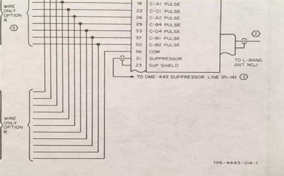
TDR-90 Interconnect Wiring Diagram, Pro Line II, ARINC 429 (With CAD-870), Single Installation Figure 2-3
