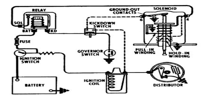
Overdrive Electrical Circuit Wiring Diagram
