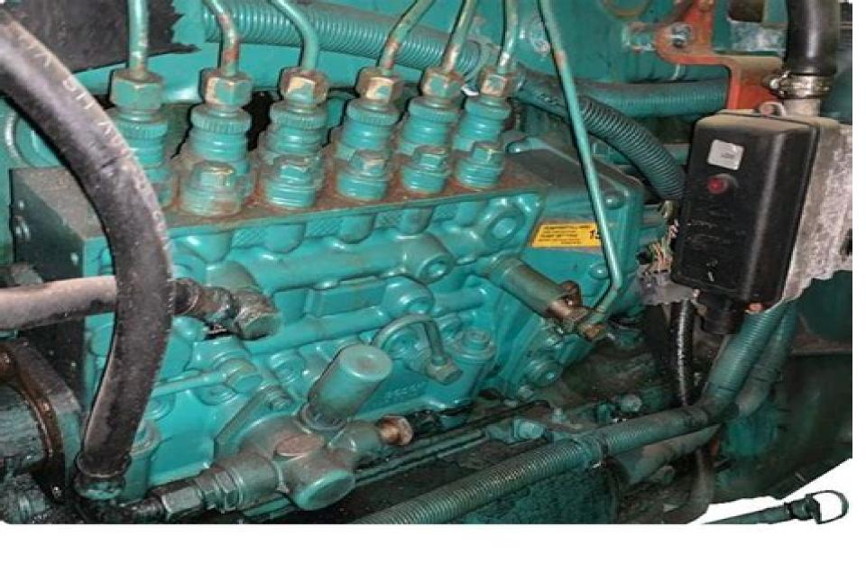
Volvo Penta TAMD 75 P-A 480 Hp @ 2600 RPM 353 kW @ 2600 RPM
