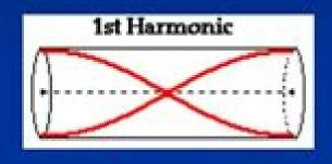
Note that the wavelength  $\lambda$  is twice the length L of the air column:
