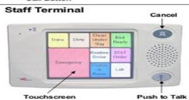
The Staff Terminal is a device that functions as a patient or procedure room communications tool while providing staff with a touchscreen to initiate an instantaneous notification of an in room need. Additionally it may be used as a functional nurse call console or duplex intercom station.
