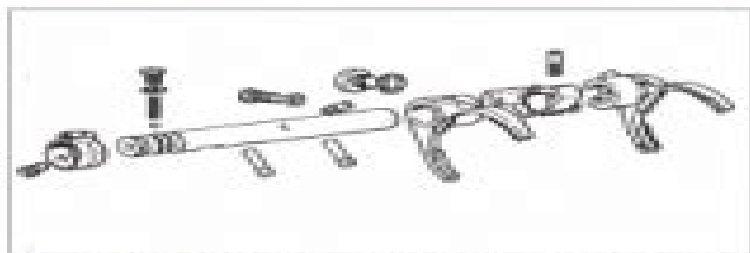
Fig. 17 - Components of inverter rod and fork as assembly for gearbox with minireduction.
