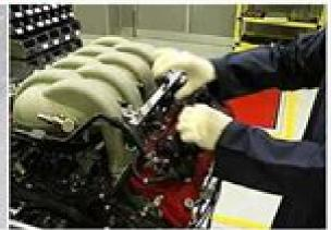
3. Remove the corrugated tubes from the wire guides.
