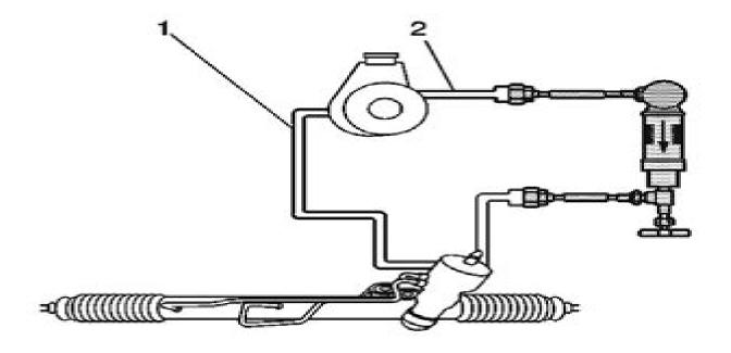
Fig. 3: Testing Rack and Pinion System Pressures Courtesy of GENERAL MOTORS CORP.
