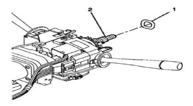
Fig. 21: Wave Washer & Steering Shaft Courtesy of GENERAL MOTORS CORP.
