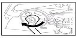
Unscrew the clutch from the crankshaft.
