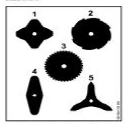
Cutting attachments 1, 4 and 5 may be mounted either way round – they must be turned over regularly to help avoid one-sided wear.
