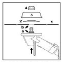
Place the cutting attachment (1) in position.
