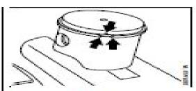
Note: One (FS 45) or two (FS 45, 55) piston ring(s) is/are used depending on the model in question.
