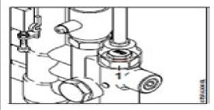
Unscrew safety valve (1) with a size 22 insert (2)
