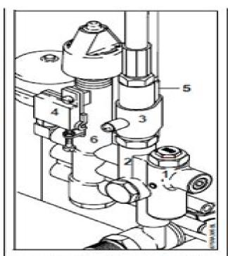
The regulation valve block can be dismantled into the following component parts in order to reach the main seals without changing the setting of the regulation valve block:
