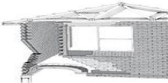
Cavity brick construction is two brick walls standing side by side separated by a cavity, tied together with brick ties that cross the cavity and embedded into the mortar joints. Floors can be either concrete slab or timber.
