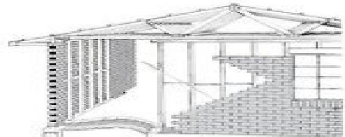
The brick walls are a facade anchored with brick ties to a timber or steel frame. The frame performs the structural load bearing work supporting the roof, ceiling and wall linings. A cavity space is provided between the frame and brick wall. This cavity acts as a moisture barrier.
