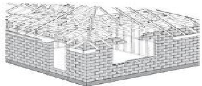
Reinforcing and grout is usually applied to specific vertical cores, lintels and a top perimeter bond beam. Walls can be cement or acrylic rendered on one or both sides or simply painted to reduce costs. Alternatively, plasterboard linings can be applied to the internal surface.
