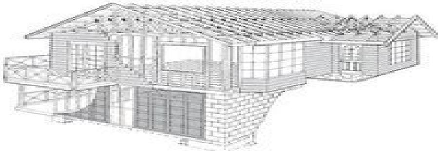
The timber framed house can be applied to one or more storeys. The external surface can be clad with timber or manufactured weatherboards and panelling, or acrylic render can be applied. Structural load bearing is performed by the timber frame.
