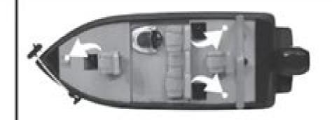
Open battery door by turning the four locks located on the battery doors.
