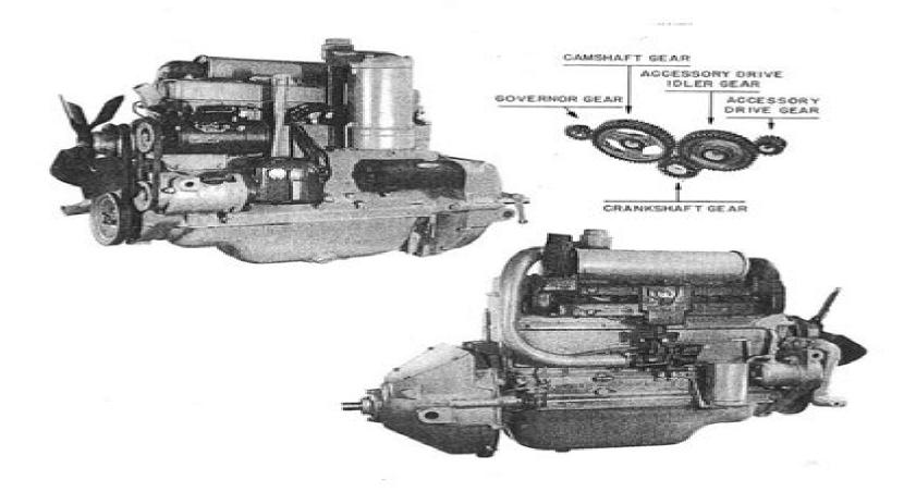
Figure 2-3-"70" HC 3-gear Engine
