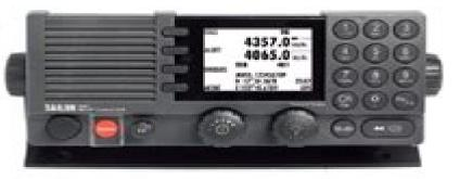
of all kinds. It offers simplex and semi-duplex SSB radiotelephony in the maritime mobile frequency bands from 150 kHz to 30 MHz. Services include voice transmissions, watch function, DSC operations (Distress calls, position info, Distress relay and more) and AM Broadcast reception.
