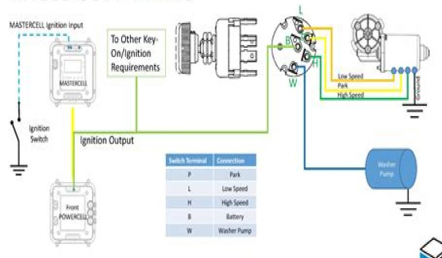
NOTE: Infinitybox Wire Colors & Connector Positions will vary for different kits. See the Configuration Sheet that came with your kit for exact wire colors and locations. Some wires omitted for clarity. Follow the instructions that came with your kit for complete details.
