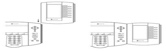
To connect up to three Expansion Modules together, repeat steps 1 and 2.
