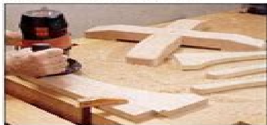
6 Use a crosscut saw to cut inclines on the top surface of the base members. Remove any cut marks by hand planing.
